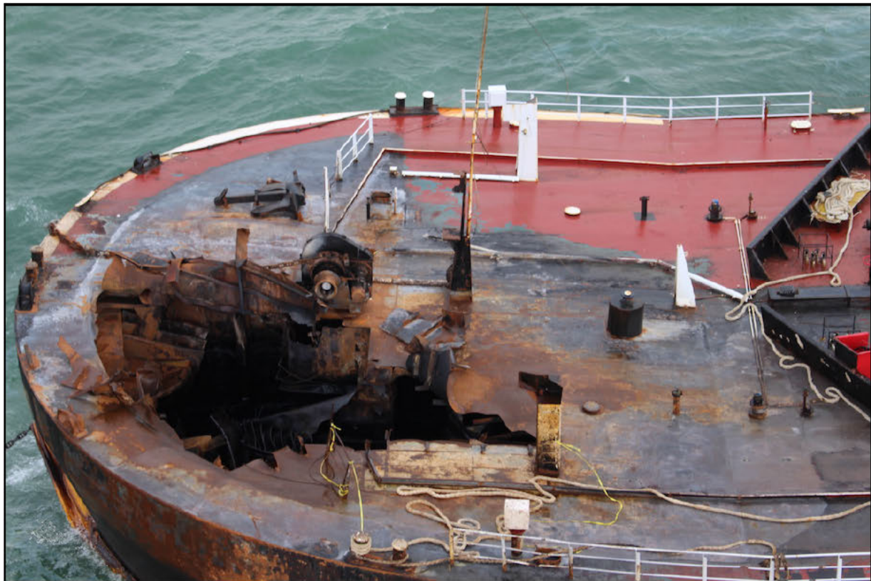
Figure 7: Overhead view of the explosion damage onboard B. NO. 255 post-explosion. Picture taken by the U.S. Coast Guard on October 22, 2017.
