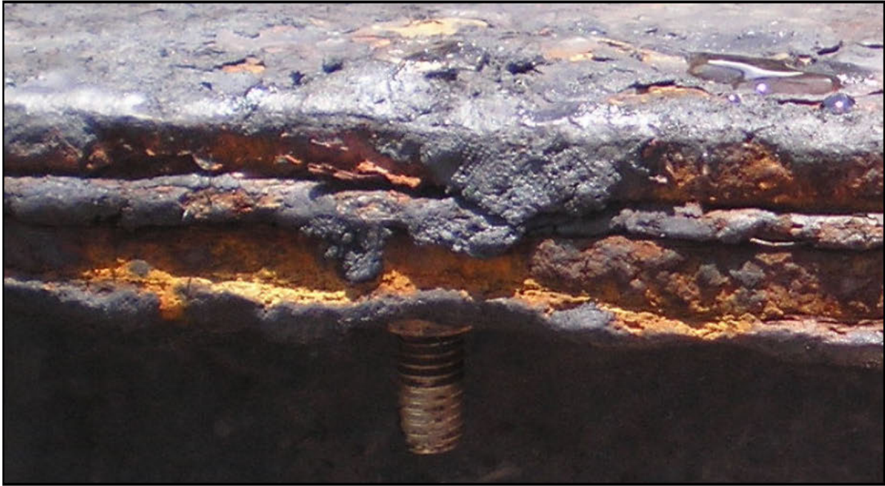
Figure 15: Close up view of the wasted cargo tank hatch in Figure 14. Picture taken by the U.S. Coast Guard in June 2018.
