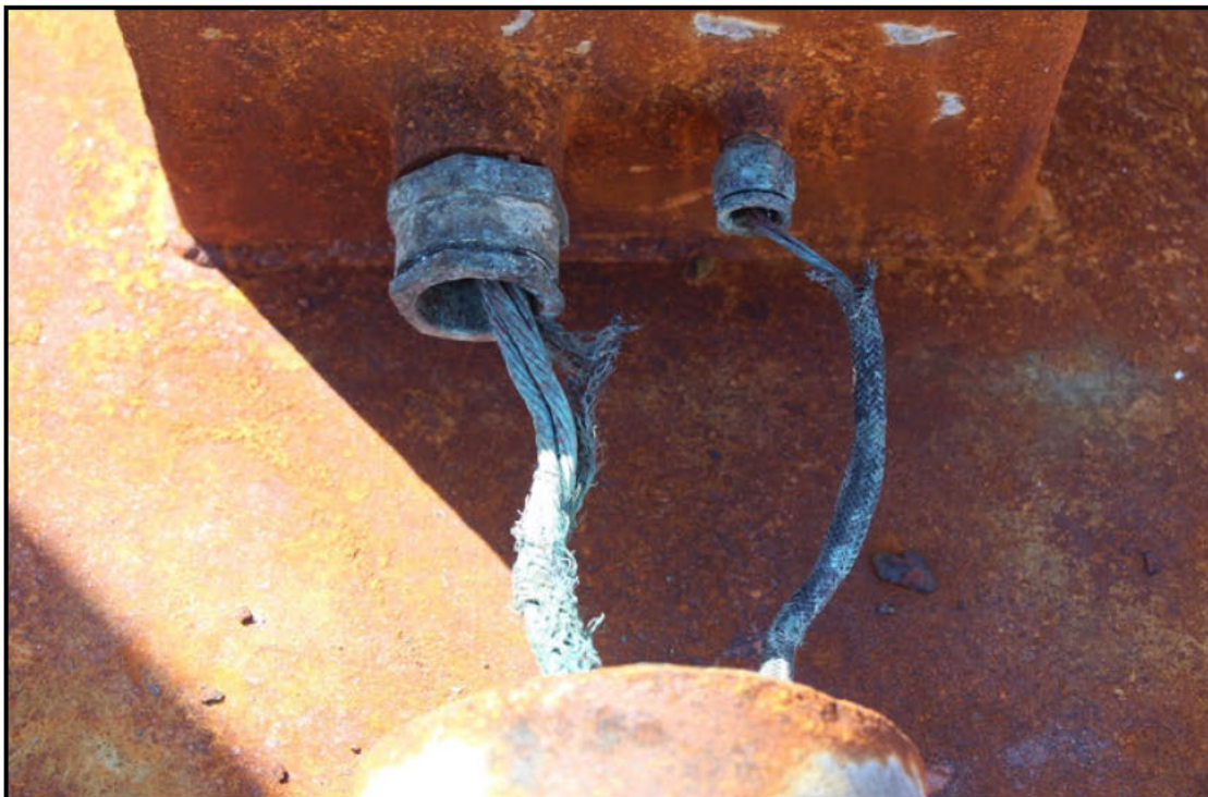
Figure 12: Deteriorated wiring located in bow area on B. NO. 255. Picture taken by the U.S. Coast Guard on November 6, 2017.
